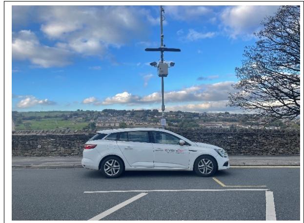
Figure 1. dBFlash system mounted on a mast with a microphone array and video camera on top for in-situ pass-by measurements.
